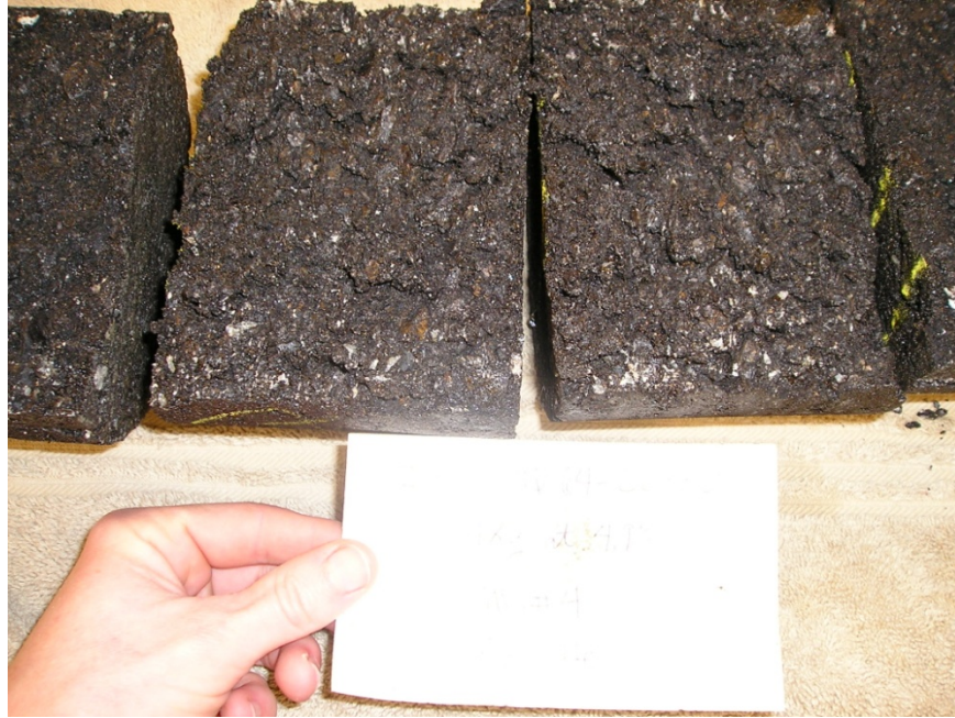
Figure 66: Unconditioned Sample, 12.5mm GMQ 64-22 with Evotherm
