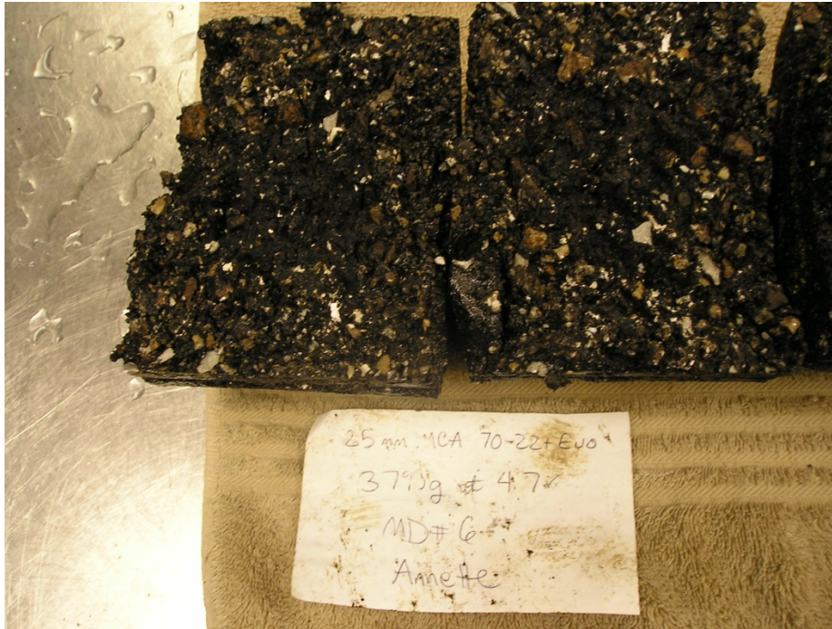
Figure 63: Conditioned Sample, 25mm MCA 70-22 with Evotherm
