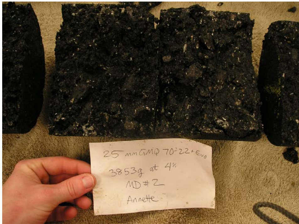
Figure 60: Unconditioned Sample, 25mm Syenite PG 70-22 with Evotherm
