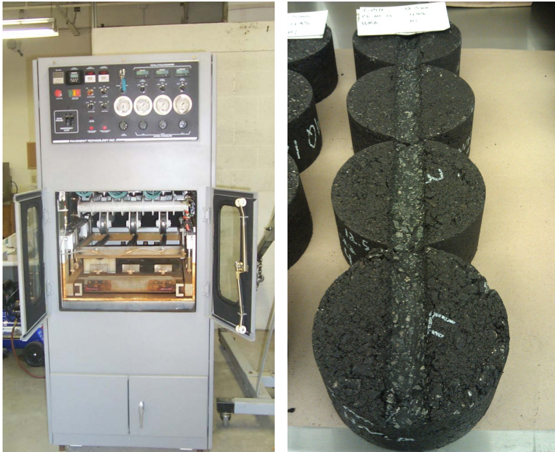
Figure 54. Asphalt Pavement Analyzer (left) and Samples after APA Testing (right)
