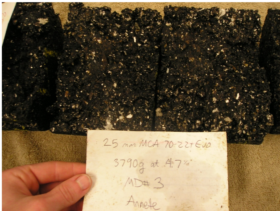
Figure 64: Unconditioned Sample, 25mm MCA 70-22 with Evotherm
