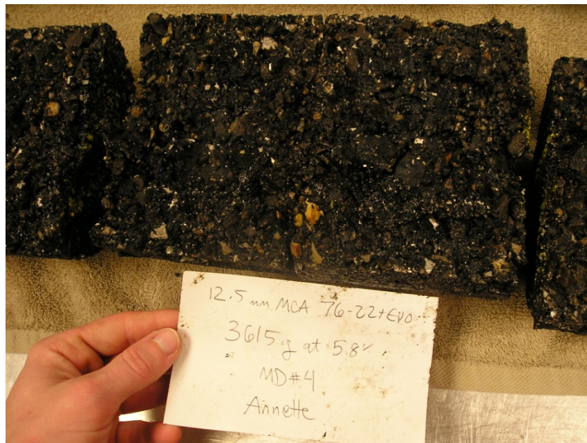
Figure 61: Conditioned Sample, 12.5mm Limestone, PG 76-22 with Evotherm
