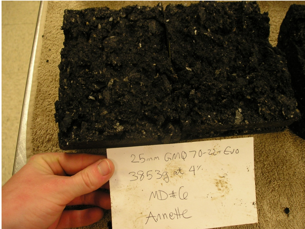
Figure 59: Conditioned Sample, 25mm Syenite PG 70-22 with Evotherm
