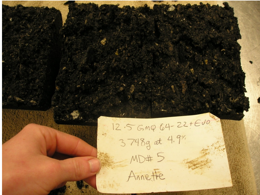
Figure 65: Conditioned Sample, 12.5mm GMQ 64-22 with Evotherm
