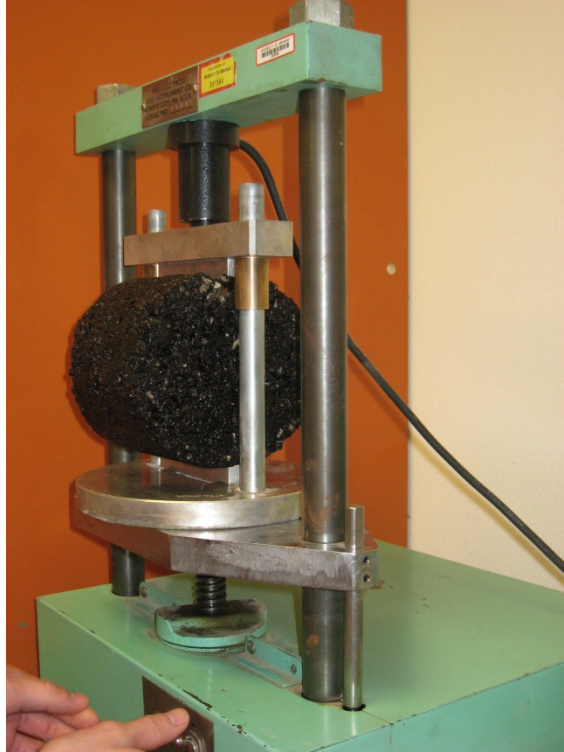
Figure 67. Load Testing in Indirect Tension Using the Modified Lottman Breaking Head
