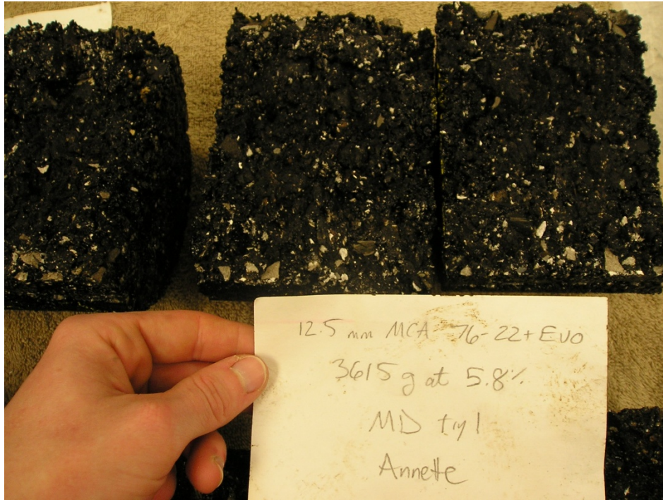
Figure 62: Unconditioned Sample, 12.5mm Limestone PG 76-22 with Evotherm
