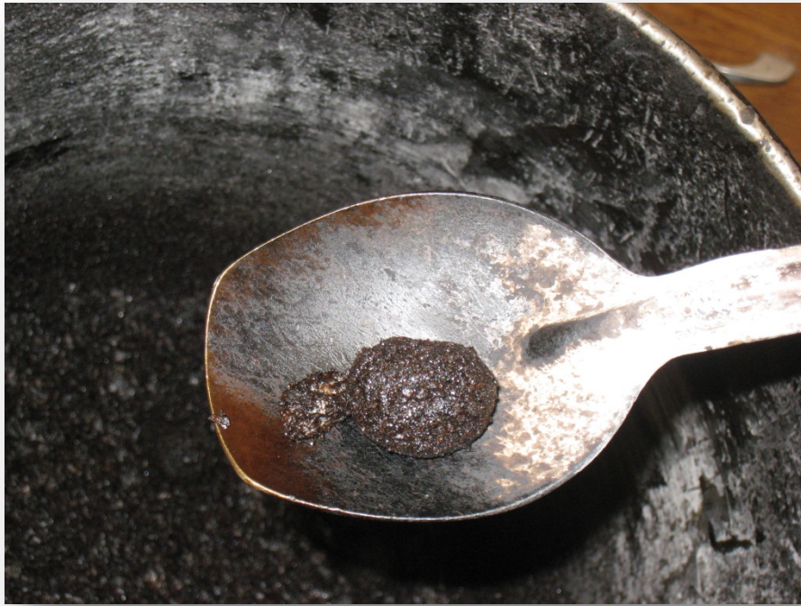
Figure 6. Binder Clumping when Maximum Temperature Reduction was Exceeded.
