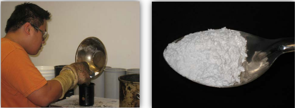
Figure 4. Addition of Advera During the Mixing Process
